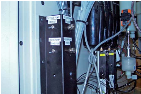
Coating pump height control and manual on off switches. The Spindles assembly must be raised before these switches will work. Its best to jog the cups away from the fountain path in case you over drive the pumps and contaminate the vacuum cups.
