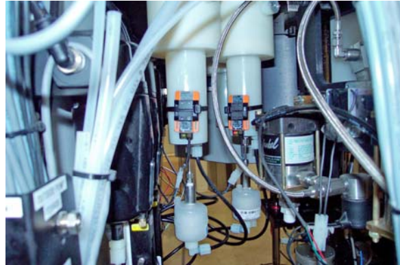
Coating bowl reservoir. Messer filters are located below the tanks. The Orange sensors are used to warn if coating is getting low.
