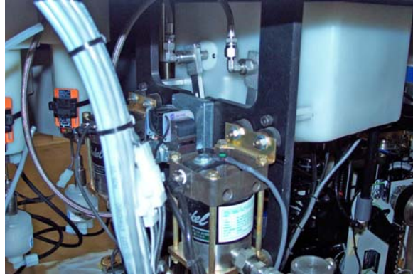
Back side of the wash tank. The wash pumps are visible, and the stainless water lines connected to the nozzle bars. The motor driving the cam to rotate the nozzles bars can also be seen.
