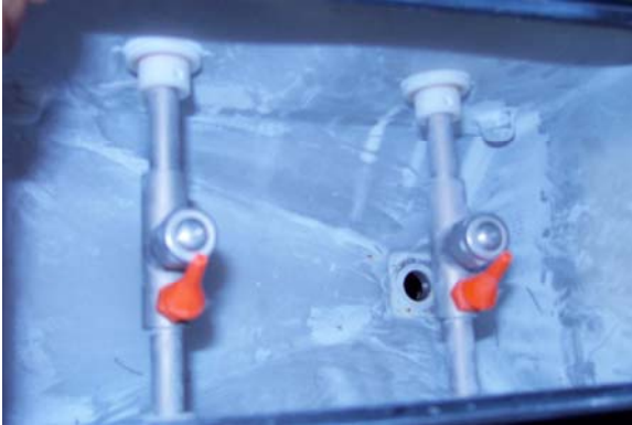
Inside of cleaning tank. The silver nozzles are the high pressure water outlets. The orange nozzles are the air dry outlets.
